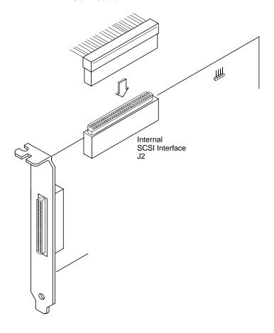
Step 2. Plug the 68-pin connector on the other end of the internal SCSI ribbon cable into the SCSI connector on your internal SCSI device. An example of this connection is shown in Figure 2.5. You must match pin 1 on all connections.
